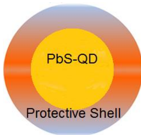
Figure 3. Schematic of a PbS-QD with a PS
