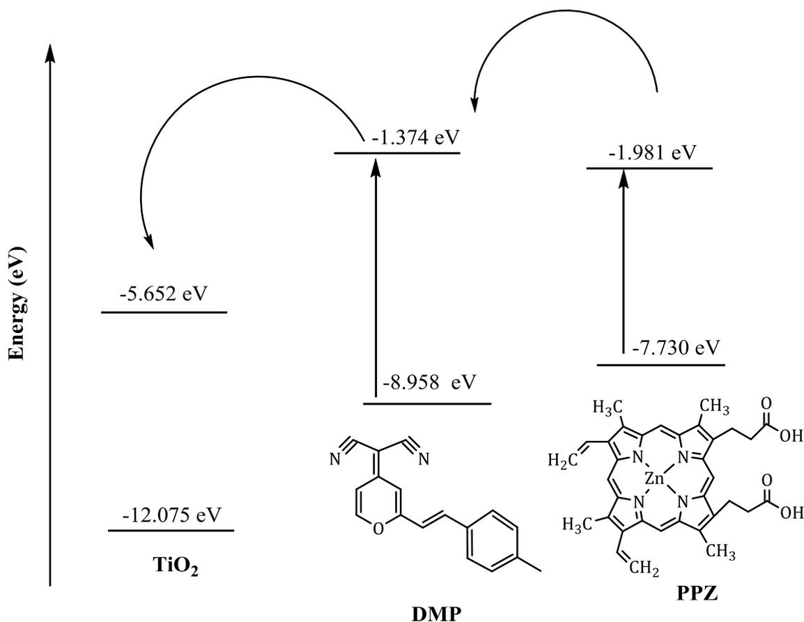
**Scheme 1.** The chemical structures of protoporphyrin IX zinc (II). (PPZ) 4-(dicaynomethylene)-6-(P-methylstyryl)-4*H*-pyrane (DMP) and the flow of electron from PPZ to  $\text{TiO}_2$  in a cascade manner based on their  $E_{\text{HOMO}}$  and  $E_{\text{LUMO}}$  values
