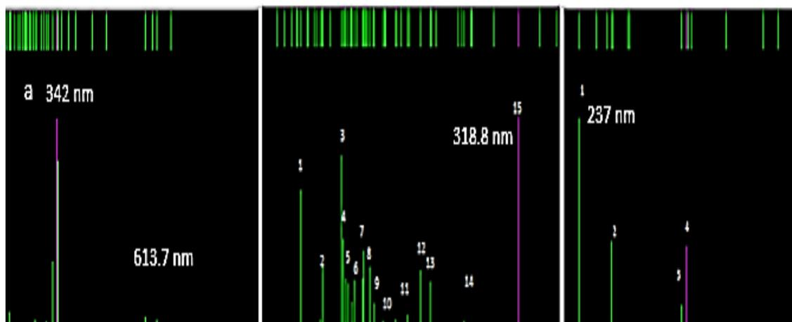
**Figure 4.** Electronic absorption spectrum of a) PPZ, b) DMP and c) TiO<sub>2</sub> determined using ZINDO/s option of semiempirical method
