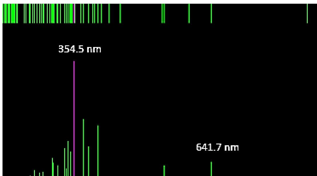
**Figure 5.** The theoretical electronic absorption spectrum of PPZ-TiO<sub>2</sub>
